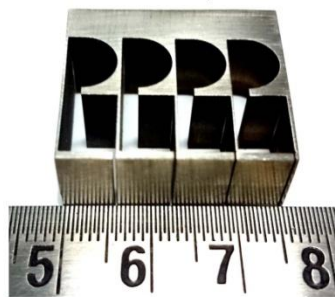
Profile slot through Inconel 706 plate
