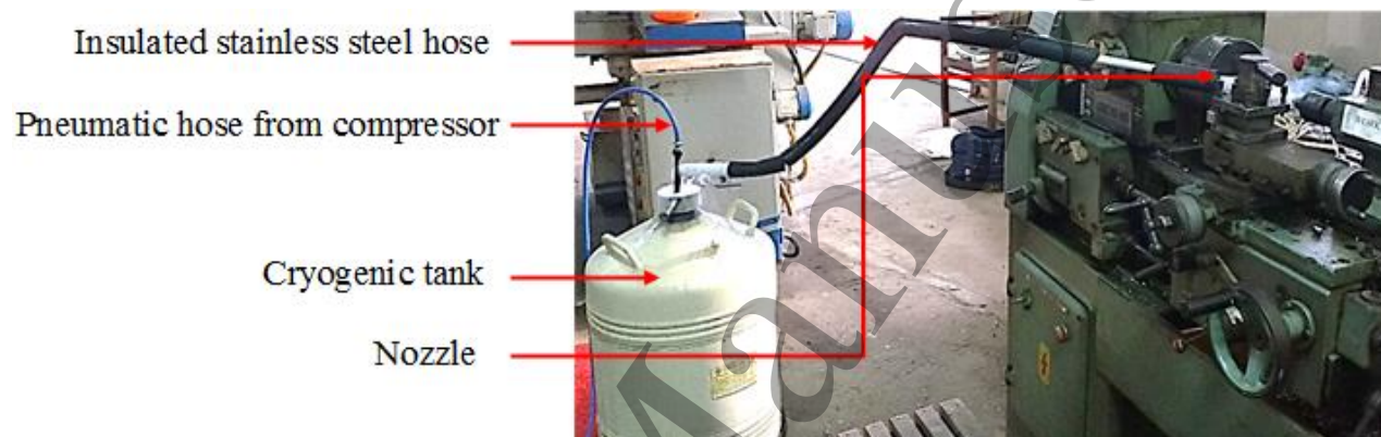
Figure 1. Cryogenic diamond burnishing setup
