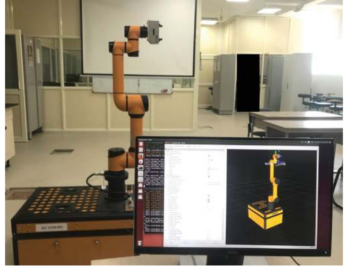
Figure 3. Photo of the JR2 mobile manipulator along with its kinematic control package, namely, the MoveIt software in the lab environment.
