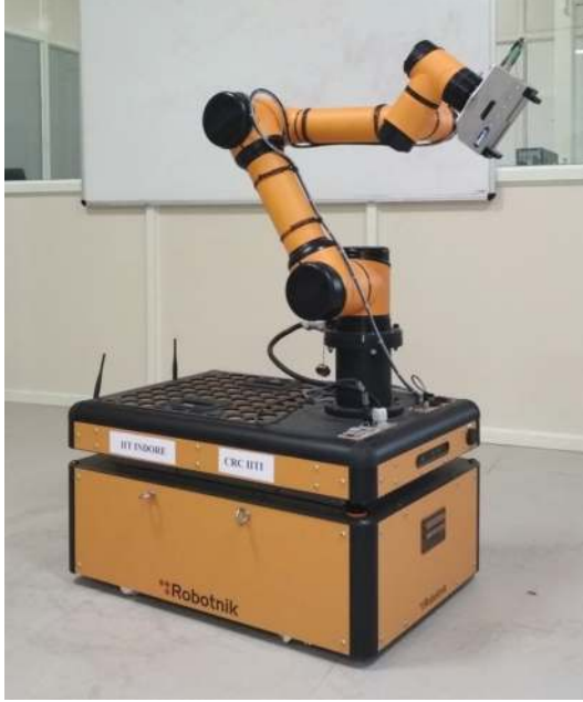
Figure 1. Photographic image of the JR-2 vehicle-manipulator in lab environment.
