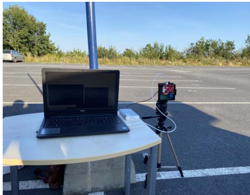
Figure 2. The mmWave radar measurement setup.
