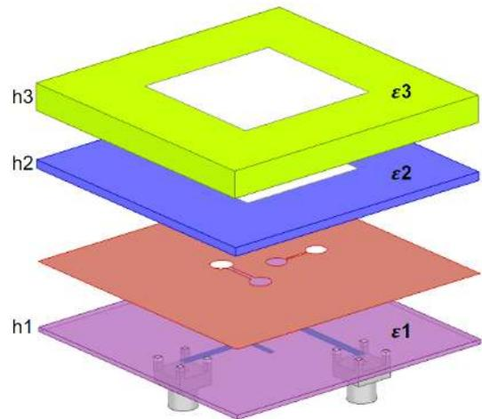
FIGURE 1: Expanded view of the antenna element
