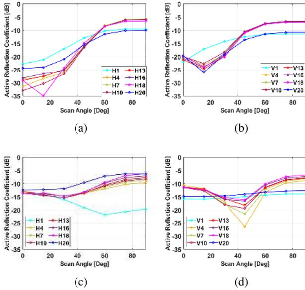
FIGURE 9: Active S-Parameters for some of the (a) H and (b) V Ports at  $d=0.5\lambda$  and for (c) H and (d) V Ports at  $d=0.4\lambda$  of a 2X20 Array at 2.8GHz
