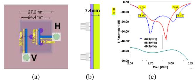
FIGURE 2: (a) Bottom view of the antenna element (b) Side view of antenna element (c) S-parameter plot
