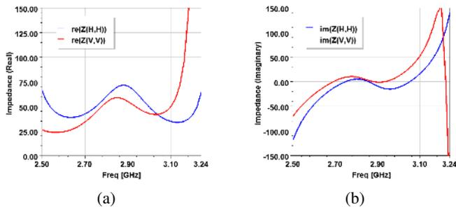
FIGURE 4: (a) Real and (b) Imaginary Impedance plots of single element
