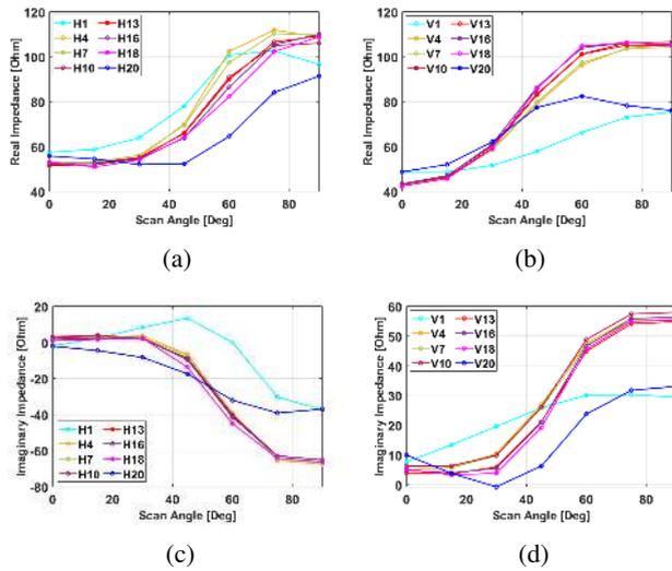
FIGURE 13: Active Z-Parameters for some of the (a) real (Z) H and (b) real (Z) V (a) imag (Z) H and (c) imag (Z) V of 2X20 Array at 2.8 GHz and  $d=0.5\lambda$
