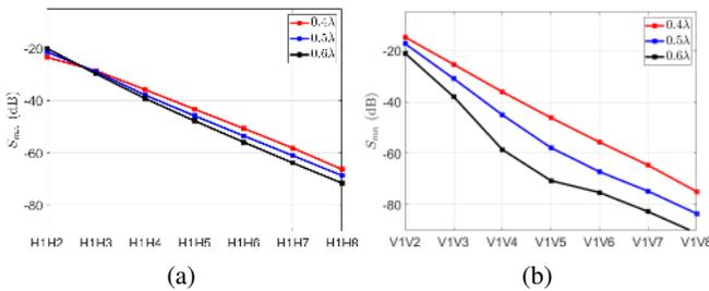
FIGURE 8: Mutual coupling effects for (a) H and (b) V Ports for 2X20 Array at 2.8 GHz for  $d=0.4\lambda$ ,  $d=0.5\lambda$  and  $d=0.6\lambda$
