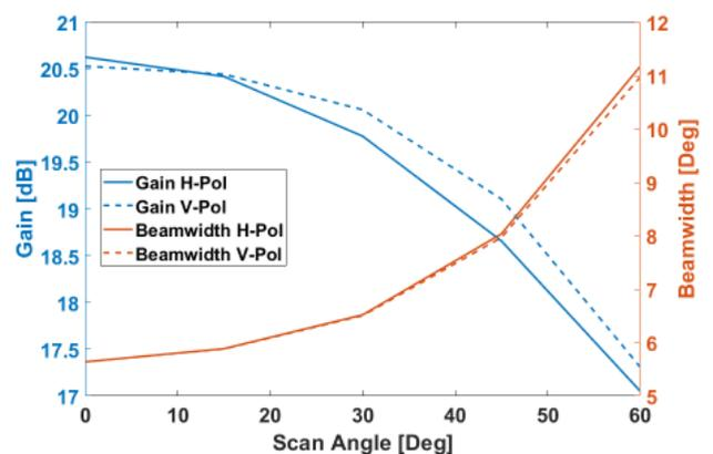
FIGURE 7: Variation in gain and beamwidth of the 2X20 array with scan angle
