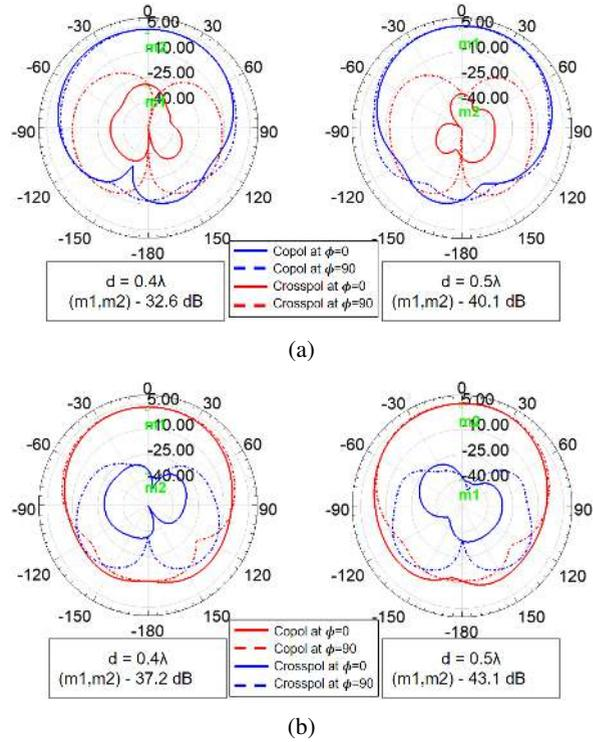
FIGURE 12: Active element patterns for  $0.4\lambda$  and  $0.5\lambda$  spacing for (a) H and (b) V polarizations
