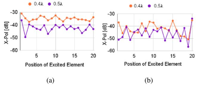
FIGURE 14: Cross-polarization level of active element patterns at different positions in the array for (a) H and (b) V polarizations
