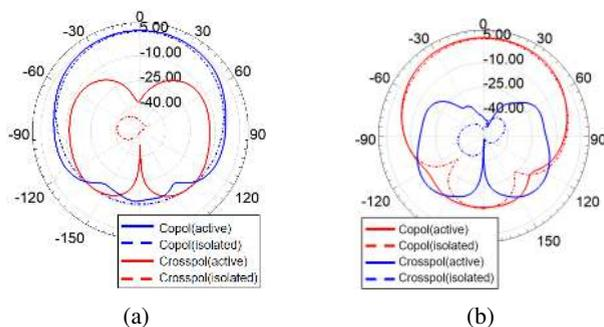
FIGURE 11: Active element patterns and isolated element patterns for (a) H and (b) V-polarization
