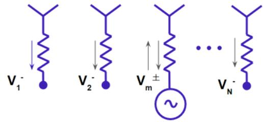
FIGURE 10: Schematic view of array of N elements with only  $m^{th}$  element excited
