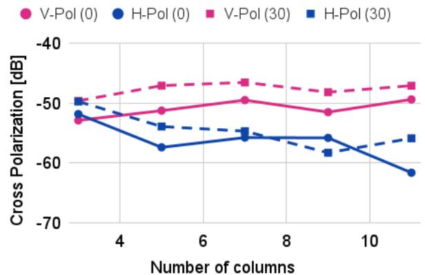
FIGURE 15: Cross-polarization level for different scan angles for the 2X20 array
