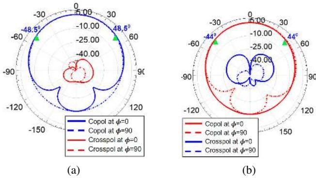
FIGURE 3: Gain pattern with (a) H port excited and (b) V port excited
