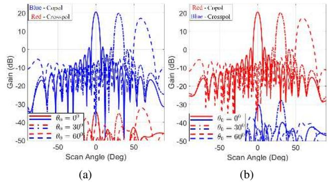
FIGURE 6: Gain pattern for a 2X20 array with (a) H and (b) V polarization and spacing =  $0.5\lambda$
